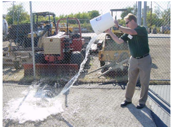
Joe Krueger demonstrates the amazing pervious concrete sample. Pervious concrete can hold up to 4" of water in an hour.
